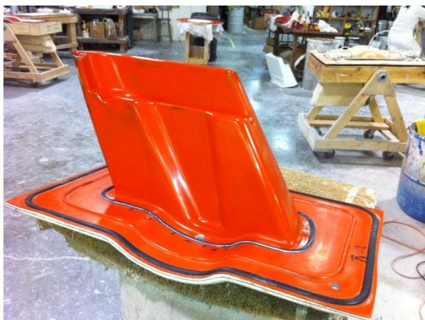
**XTEND® 19RSS provides easy release and reduces scumming and buildup on “B” sides in RTM.**
